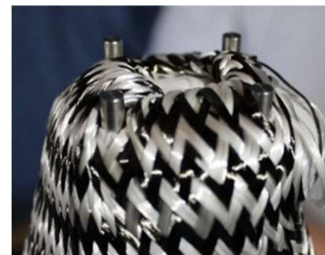
(Fig 2: example of loose tie off of braid to facilitate full fabric saturation)
